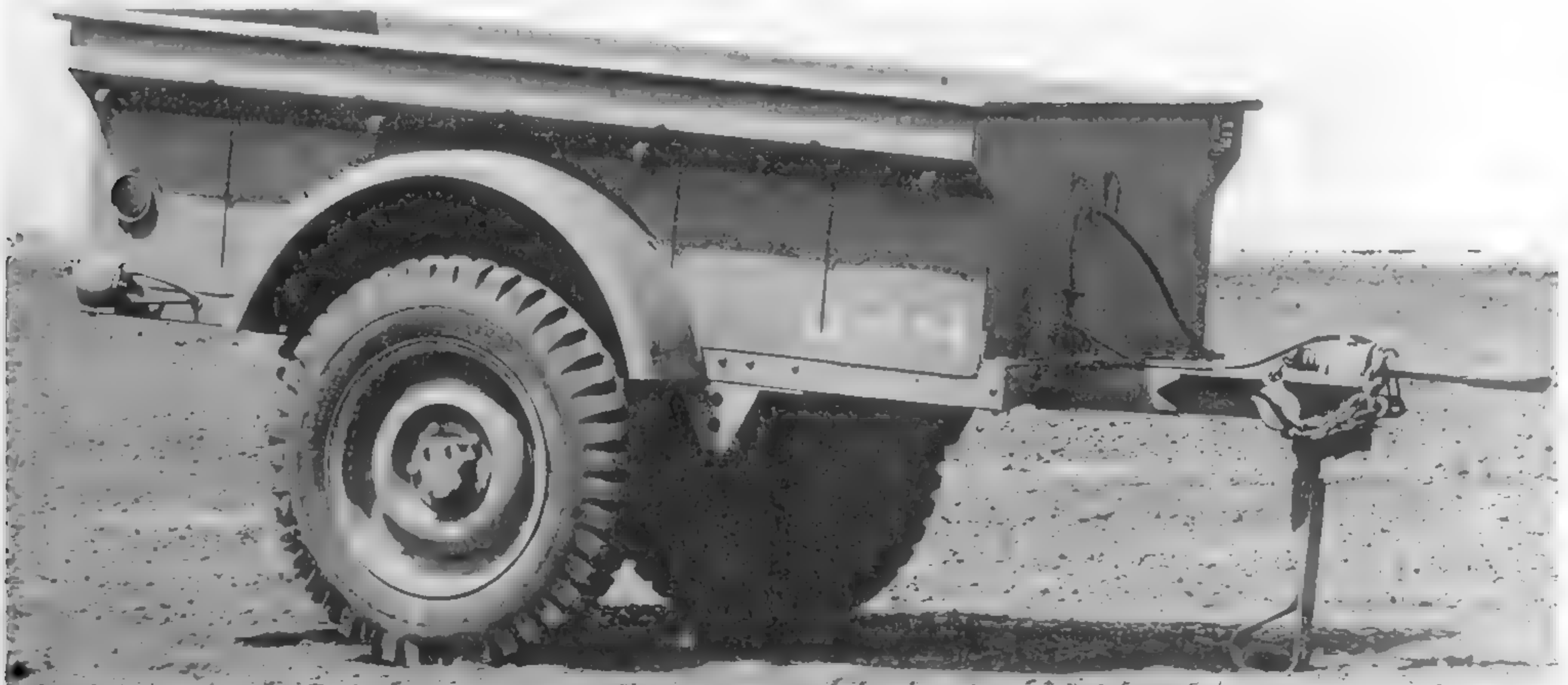
This June 1945 Studebaker Proving Ground photo shows a factory-fresh Bantam 1/4-ton trailer. Notice the style of parking brake handle and lack of handgrips on the corners of the bed. These are the characteristics that most readily distinguish the WWII vintage trailer from the postwar M100. (U.S. Army photo)
